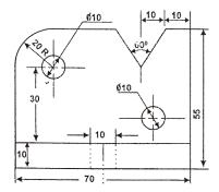
**3.** Draw the auxiliary view of the slopping surface of the object shown in the following figure :
