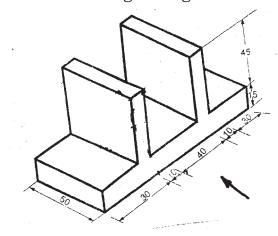
**4.** Draw the auxiliary view for the given orthographic views as shown in below.
