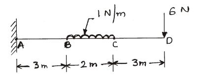
**15.** Draw shear force and bending moment diagrams for a simply supported beam shown in the figure below :
