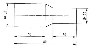
Work material: mild steel, work size: 32 mm dia, length: 90 mm, speed: 800 r.p.m., feed 200 mm/min. Depth of cut 2 mm. Assume all other data.
