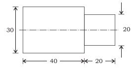
Cutting speed = 600 r.p.m. Feed = 1.50 mm/min Depth of cut should not exceed 2 mm
