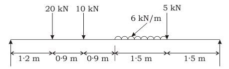
**15.** Draw shear force and bending moment diagram of given cantilever beam :
