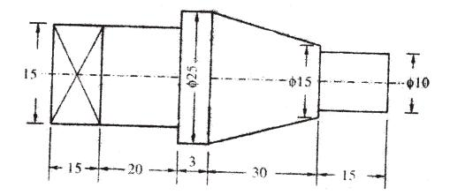
14. The shaft shown below is to be manufactured by turning out of 85 mm steel rod. Find out the minimum machining time if the job is to be turned at 300 r.p.m. with feed 0.5 mm/rev and depth of cut 3 mm. All dimensions are in mm:
