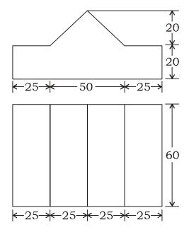
**9.** Draw the front view and top view of the given figure in first angle projection.
