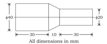
Take cutting speed = 800 r.p.m. Feed = 200 mm/min Depth of cut = 2 mm
