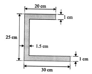
(b) Calculate the Moment of Inertia of the area shown in the fig. about horizontal centroidal axis.
