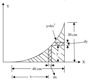
5. Calculate the moment of inertia of the section shown below about the XX and YY axis through the centroid.
