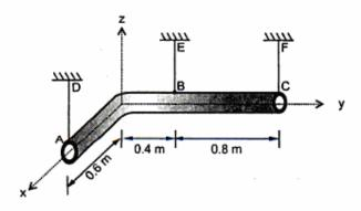
b) Calculate the magnitude of the force supported by the pin at B for the bell crank (8M) loaded and supported as shown.
