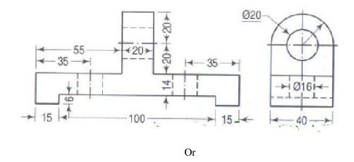
10. Draw the (i) Front view (ii) Side view (iii) Top view for the following Figure. (15M) All dimensions are in mm.
