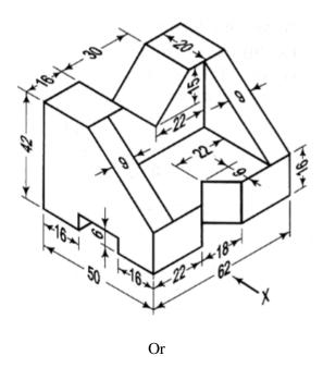
10. Draw the isometric view of the following figure. All dimensions are in mm.
