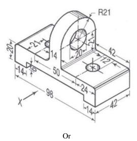
10. Draw the isometric view for the figure 1 shown below front and top views. All (15M) dimensions are in mm.
