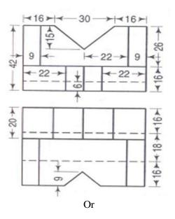
10. Draw the orthographic view of the following figure. All dimensions are in mm. (15M)
