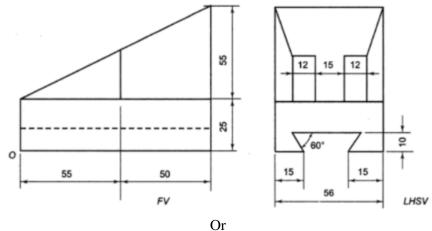
Draw the elevation, top view and side view of the following machine part as shown in Fig.1below. (All dimensions are in mm.)
