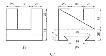
Draw the elevation, plan and left side view of the object given below. (14M)
