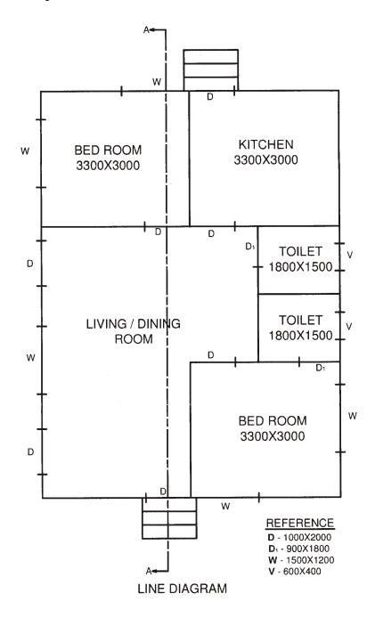
*(iv)* Superstructure : All the walls are 200 mm thick except partition wall between toilets which is constructed on the floor with thickness of 100 mm. The height of walls is 3300 mm to the bottom of RCC roof slab.
