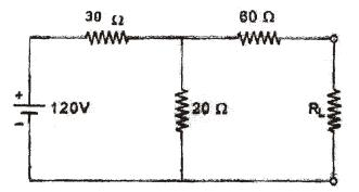
(b) Using Norton's theorem, find the current in the load 5 resistance  $R_L$  of the circuit shown below.
