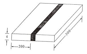
Filler rod diameter = 3 mm Filler material lost during welding = 20% Oxygen consumed =  $0.55 \text{ m}^3/\text{hr}$   $C_2H_2$  consumed =  $0.27 \text{ m}^3/\text{hr}$ Filler rod length consumed = 3.4 m/m of weld Welding time/meter of weld = 20 min Density of filler material = 7.2 gm/ccCost of filler material = ₹ 45 per kgCost of oxygen =  $₹ 30 \text{ per m}^3$ Cost of acetylene =  $₹ 150 \text{ per m}^3$
