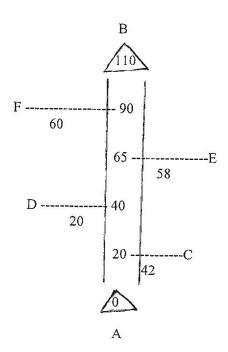
**14.** The following perpenducular offsets were taken from a chain line to a curved boundary line :
