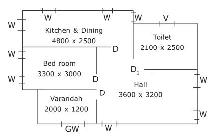
All dimensions are in mm, all walls are 200mm thick in superstructure.
