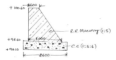
9. An RCC square column footing of a overhead tank as shown in figure. Calculate the cement concrete quantity for the footing.
