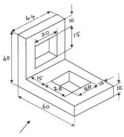
**9.** Draw the isometric drawing of an object whose orthographic projections are given below:
