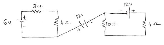
/4457 2 [Contd... WWW.MANARESULTS.CO.IN **12.** Use Thevenin's theorem to find current through 5 ohm resistor in the circuit shown below :
