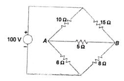
**13.** Find the load impedance required to be connected across the terminals *A*-*B* for the maximum power transfer, in the network shown in the figure below. Also find the maximum power delivered to the load :
