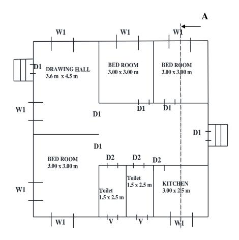
7. Draw the line diagram of a Apartment Plan of the Floor with 6 Units each@ 90 to 120 sq.m.15 m
