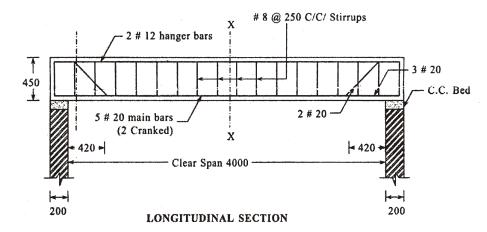
**5.** Prepare the bar bending schedule and find the total quantity of steel required for the one-way slab shown below. Assume all covers as 20 mm:
