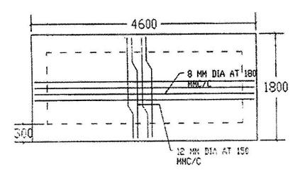
Thickness of slab = 100 mm All the covers = 20 mm
