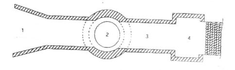
5. The abutment of a surplus weir has a top width of 0.75 m. TBL is +62.000. Top and bottom level of cc bed are +57.800 and +57.350 respectively. The abutment has a batter of 1 in 4 at water face and 1 in 6 at rear face. Offset of cc bed is 0.30 m on either side. Draw the cross section of the abutment.
