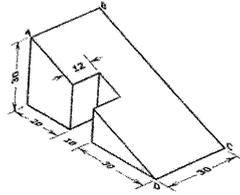
4. Draw the auxiliary view for the inclined surface of the following object :
