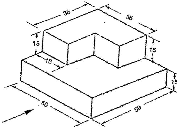
9. Draw the isometric view of the ribbed angle plate shown in figure below. All dimensions are in mm and the views are given in the first angle :
