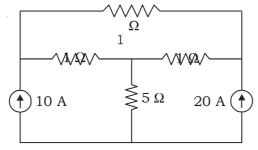
14. Obtain Thevenin's equivalent circuit for the bridge circuit shown below.
