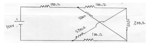
**13.** (a) Find the value of  $R_L$  in the circuit for Maximum Power Transfer and also calculate Maximum Power.
