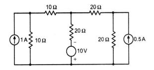
3. Write the mesh current equations for the given circuit below and arrange them in matrix form.
