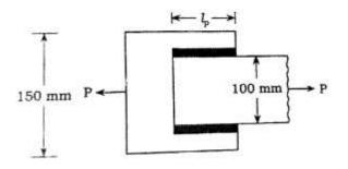
13. (a) A motor shaft of 60 mm diameter transmits a torque of 150 N-m. It has an extension of 75 mm. The permissible shear and crushing stresses for mild steel key are 55 N/mm<sup>2</sup> and 110 N/mm<sup>2</sup> respectively. Justify whether the length of key way is sufficient or not.
