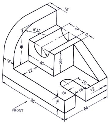
8. Draw the isometric view of a following block. (All dimensions are in mm).
