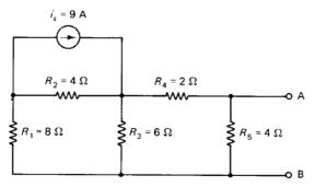
6. For the circuit shown in figure find (i) y-parameters (ii) the expression for input (16M) impedance
