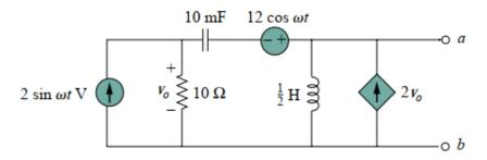
b) Find the Maximum power transfer to the load resistance, 4  $\Omega$  across *a-b* in the (8M) following circuit.
