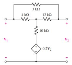
b) The two-port networks of the following figure are connected in series. (i) (8M) Determine the impedance parameters for the series connection by first finding the z-parameters of the individual networks. (ii) If the two networks are instead connected in parallel, determine the admittance parameters of the combination by first finding the y-parameters of the individual networks.
