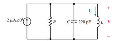
Suppose the circuit has a resonant frequency of 800 kHz and a bandwidth of 25 kHz.
