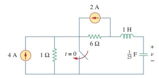
b) In the circuit shown in the following figure, the switch moves from position 1 to (8M) position 2 at t = 0. Use Laplace transforms to find v(t) for t > 0.
